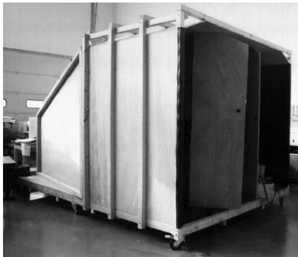
Plate 2. Exterior view of the study and design simulator for train driving.
